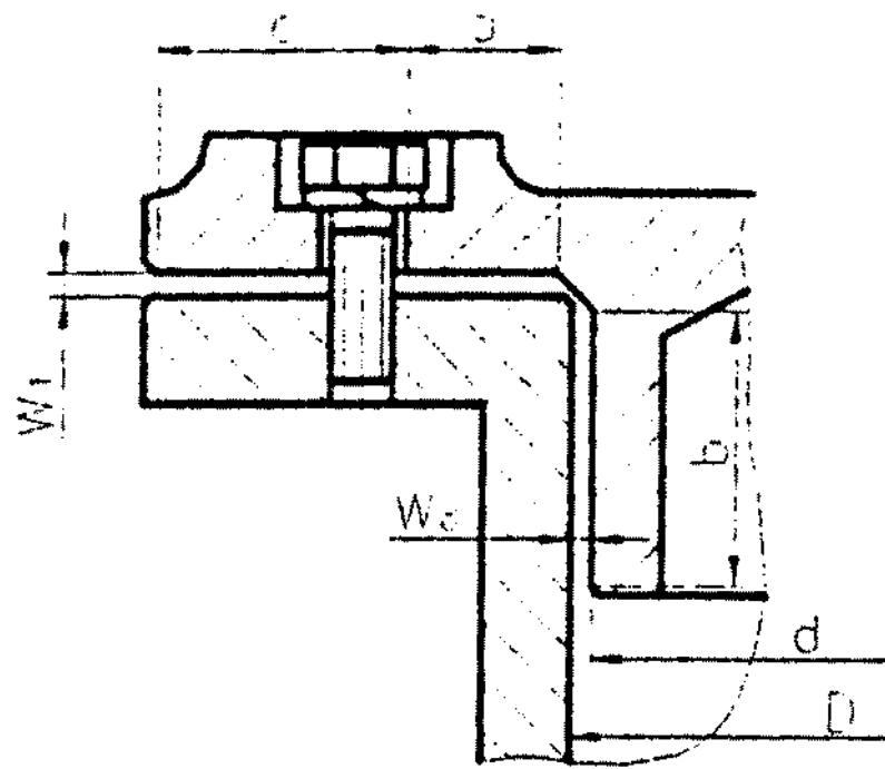
$$\begin{aligned} Wd &= D - d \\ L_1 &= b + a + c \\ L_2 &= b + a \end{aligned}$$
